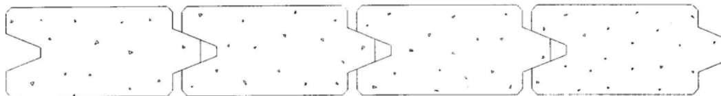
FIGURE 12-4 Concrete sheet piling
