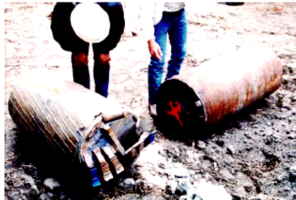
FIGURE 6-5 Drilling bucket/cleanout bucket comparison
