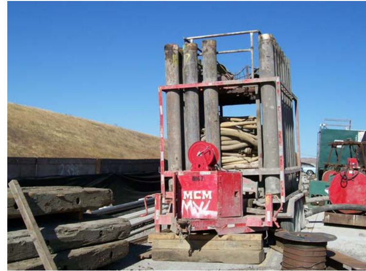
4-inch tremie tubes.
