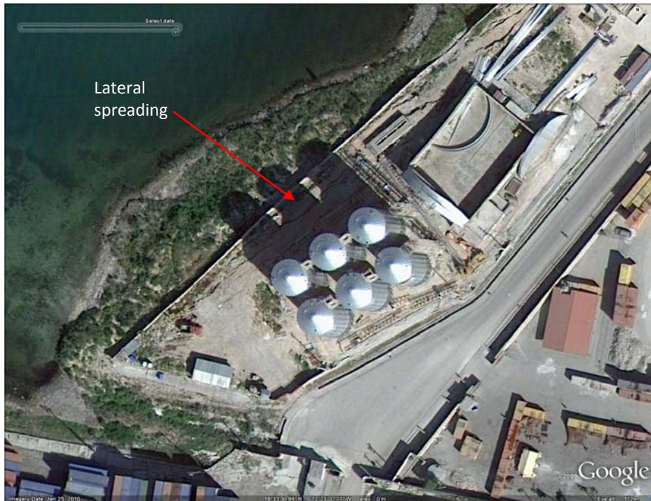
**Figure 6.18** Lateral spreading behind (westward side) steel grain hopper silos. However, the foundation system for the silos showed no visible signs of distress.
