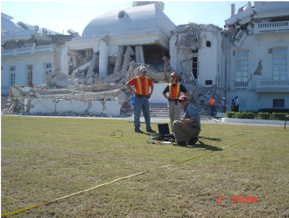
**Figure 5.9** The Presidential Palace lies within the heavily damaged zone noted above. Two SASW tests and one H/V Spectral Ratio test were conducted here (N 18.543633°, W - 72.338905°).
