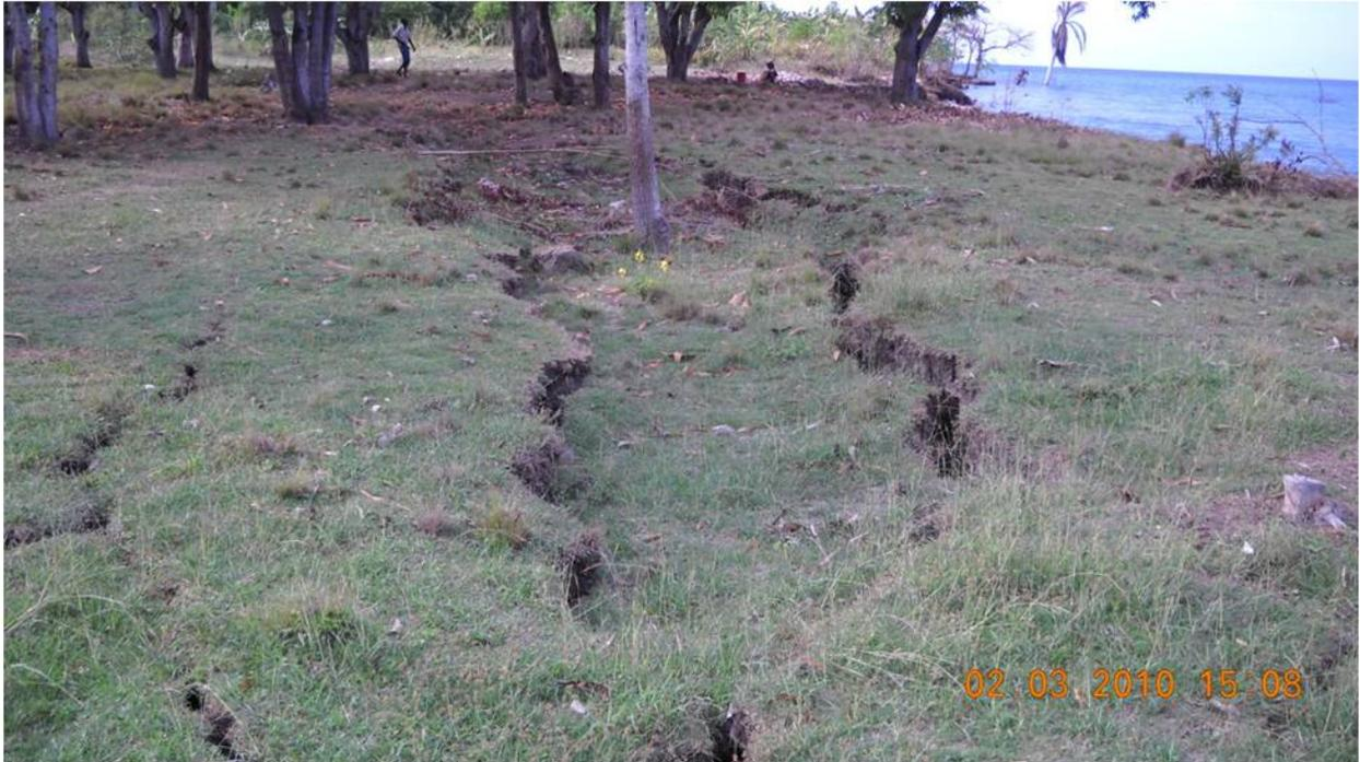
**Figure 7.19.** Graben formation subparallel to coastline at coastal failure near village of Grand Goâve. ( $18^{\circ}25'54.43''\text{N}$ ,  $72^{\circ}45'37.99''\text{W}$  looking northwest).
