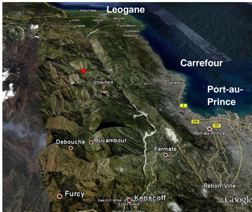
**Figure 3.1.** View west of Enriquillo Plantain Garden fault zone. Fault extends west-southwest from Pétion-ville along the prominent linear valley of the Frorse and Momance rivers at center of picture. Epicenter of 12 January M 7.0 earthquake shown by red star. The rupture extended west from the epicenter, away from Port-au-Prince.
