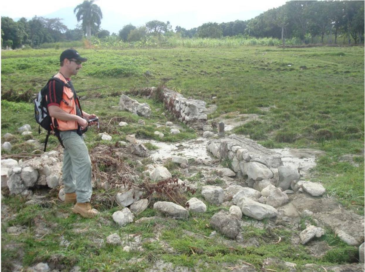
**Figure 7.21.** Sand blow formation along inland extent of coastal failure near village of Grand Goâve. ( $18^{\circ}25'53.73''\text{N}$ ,  $72^{\circ}45'37.65''\text{W}$ )
