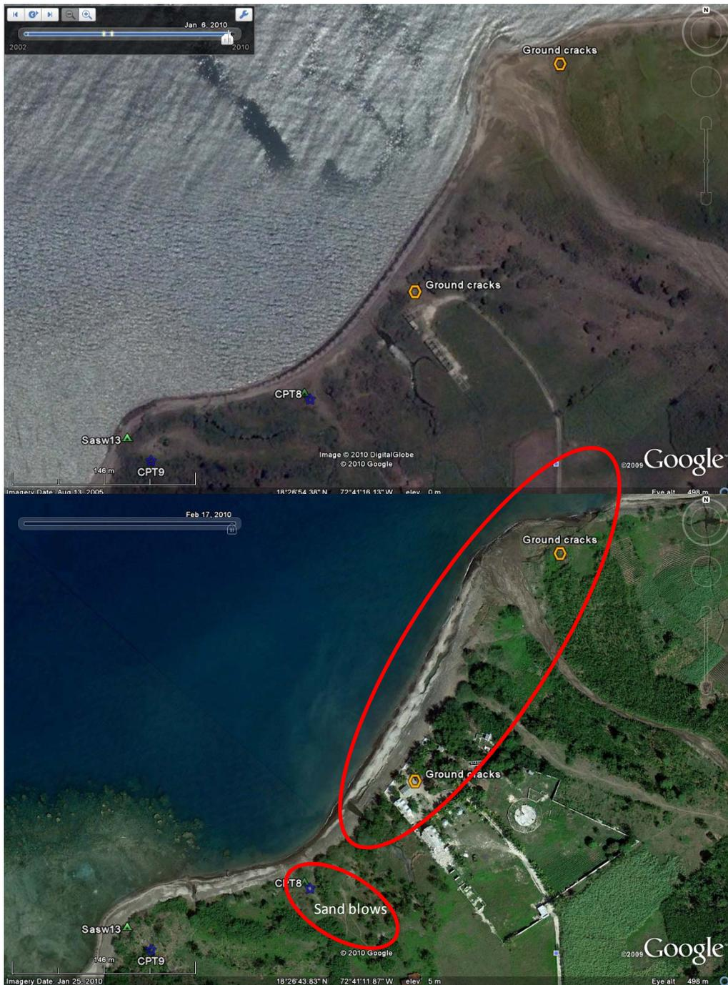
**Figure 7.3.** Pre- and post-earthquake images of coastline near village of L'Acuil. Note in the lower, post-earthquake image the significant cracking subparallel to the coast and the arcuate slump in the northern end of the failure. SASW and DCPT testing was performed near several large sand blows located near the south end of the failure zone, as well as farther south outside of the failed reach. Imagery courtesy of Google Earth. Approximate center of image at 18°26'51.17"N, 72°41'11.06"W.
