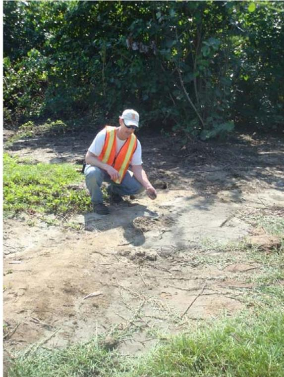
**Figure 7.6.** Sand blow formation to the south of the main cracks along coast near village of L'Acuil. ( $18^{\circ}26'44.27''N$ ,  $72^{\circ}41'12.05''W$  looking south).
