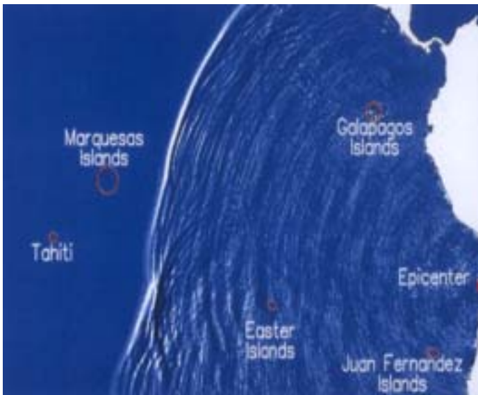
Model of the tsunami propagation in the southeast Pacific, nine hours after its generation. Source: Antofagasta, Chile (30 July, 1995)
