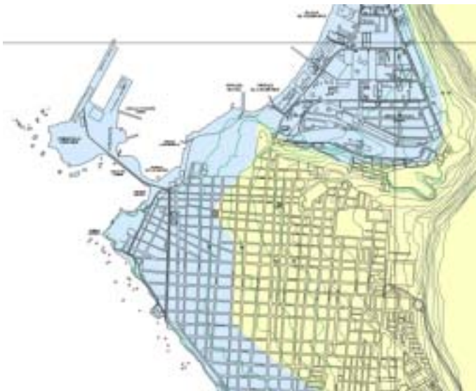
Estimated Tsunami Inundation at Iquique-Chile, based on numerical model results.
